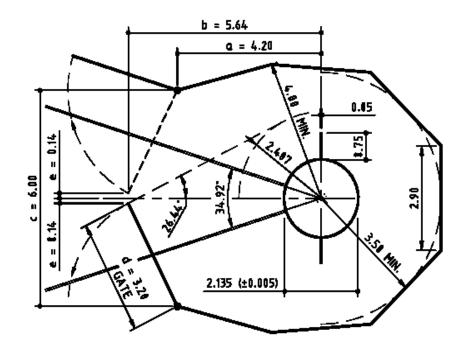
Hammer throwing cage with 3.2m gates (gate to be perpendicular to hammer throwing line) (Dimensions in m)
